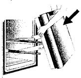
With drawer pulled out to full extension, insert lower basket by aligning tabs on both sides of lower basket with notches in rail assembly. Verify that the basket sides are hooked securely over the rails.
